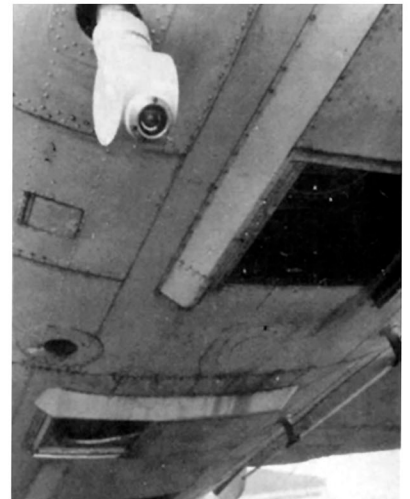
Detail shots of G-AYFA (left to right): cockpit; cabin looking forward; and belly, showing open camera ports and tracking sight
